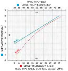
These pumps are advised for the transfer of low-high viscosity oil and similar fluids for medium-long distances. The delivery capacity of a pump varies according to particular applications and combinations. The operating pressure may vary between a minimum of 3 bar and a maximum of 8 bar.
